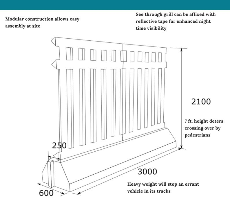
Interlocking due to the tongue & groove joint
